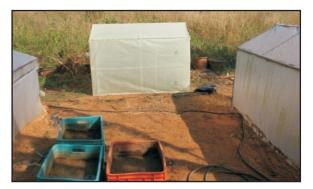
Fig. 2.3.1: Experimental set up for CO<sub>2</sub> fumigation
